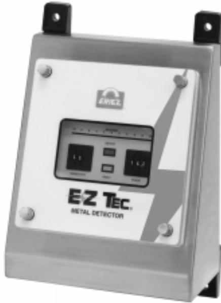
The E-Z Tec Analog Control utilizes a unique combination of digital circuitry and solid state amplifiers to process the received signal. A crystal oscillator provides a stable reference and drift free electronics and provides the user with manual selection of either WIDE ZONE detection or NARROW ZONE detection.
