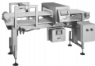
Eriez Metal Detector Conveyors may be equipped with microsized pulleys, 1/2-inch (12 mm) in diameter, to transfer small products to and from adjoining conveyors. Variable speed motors can also be provided to compensate for differing production rates and product sizes. Locking casters are also available for all conveying systems to provide easy portability.
