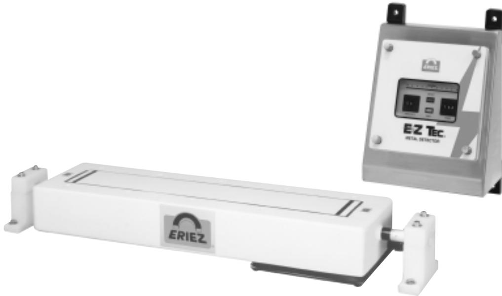
The SlimTec Single Surface Model provides highly sensitive detecting capabilities in a design effective for detecting metallic contaminants in wide, thin products. The flat-surfaced detection area is positioned beneath the product or conveyor belt. This design can accommodate materials such as sheet plastics, wood, rubber, woven materials and particle board. The SlimTec is also ideal for inspecting liquids in metal-capped bottles.
