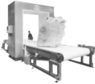
Eriez offers technical expertise when combining metal detection and customized conveying systems. Engineering experience has enabled Eriez to manufacture the largest Metal Detection Conveyor System ever built (see photo above). The 80-inch high by 66-inch wide (2032 x 1676 mm) aperture unit provides excellent sensitivity down to 0.480 inch (12 mm) steel. The stainless steel framed 30' (9 m) long conveyor can easily convey up to 2600 pounds (1200 kg) of material.
