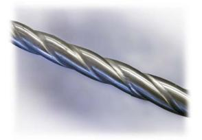
**Corrugation:** The heat exchanger surface is shaped into turbulence-inducing, alternating parallel grooves and ridges to increase heat transfer efficiency. Inducing turbulent flow results in less total surface area required to achieve the desired thermal results. Turbulent flow promotes thorough mixing of the product and even thermal disbursement without compromising product integrity.
