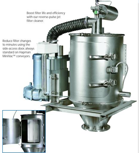
**supply.** The MiniVac<sup>™</sup> comes complete with an integral blower, eliminating the need for expensive plant air or a separate compressor.
