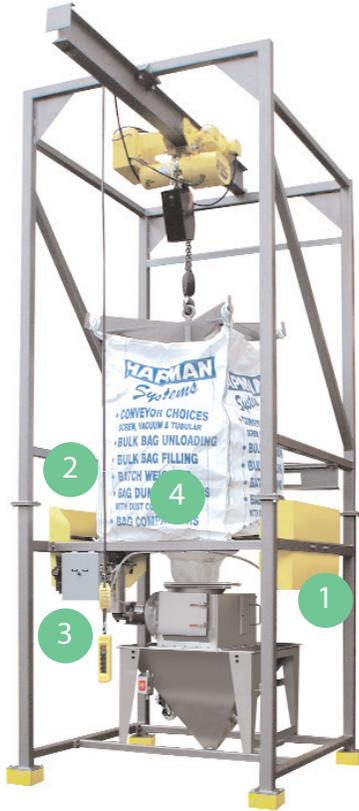
3. Batch weigh systems for gain-in-weight or loss-in-weight are accurate to one pound and allow you to perform simultaneous batching, weighing and blending operations.
